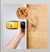
The new Termatrac system can detect insect motion behind sheetrock as well as detect moisture level spikes indicating possible insect activity. Once you have confirmation of areas of activity, then you only need to open those areas to limit repair costs.
